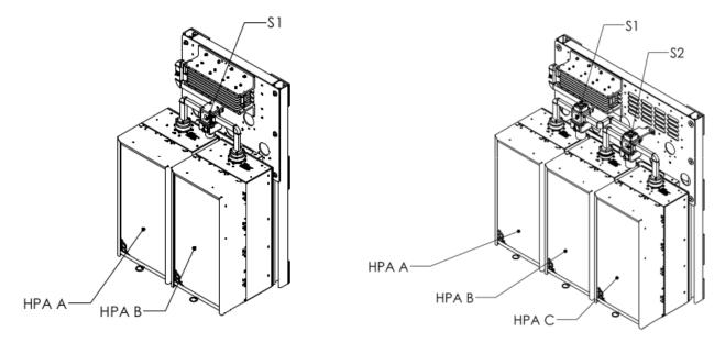
Installation of SpacePath systems and power amplifiers is easy. The light-weight, modular design enables installation by a single person, even in some of the most difficult to access applications. Simply remove the amplifier from its shipping container, install a single mounting bracket and slide into the system. Secure the waveguide quick connect then lock the bracket and plug in the cables. The amplifier is ready for a quick software configuration for the system and ready for use.
