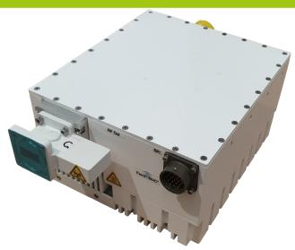
The SpacePath Communications 100W BUC / SSPB / SSPA powered by GaN technology super compact series are *revolutionary in size*, weight and power density. This series offers superior performance in an extremely compact package that can fit in your palm! Weighing at only 4.5KG, our feature-rich GaN unit is exceptionally powerful for its size: up to 100W Psat. Built in DC or AC power supply provides the customer with the simplest and least expensive plug-into-the wall solution.
